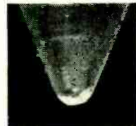
Left: Fig. 3. Fibre needle after playing one side of new 12-in record. Right: Fig. 4. Sapphire point after 250 playings of 250 new 12-in records with a "lightweight" pickup. Weight on point 25 grams.
