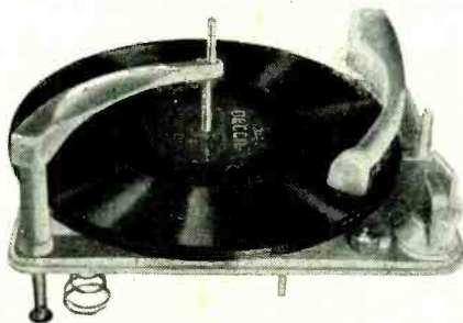
Decca record changer for standard or long-playing records fitted in the Model 92 radio-gramophone and pickup for long-playing records showing roller safety device. Pickups are colour-coded for stylus size.
